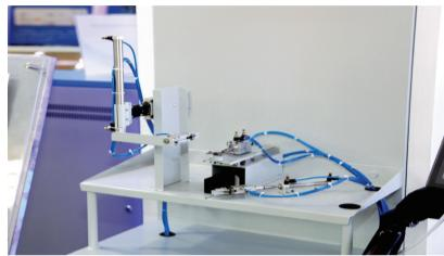
**光纤剪裁及涂料溢流承接智能机械手**
